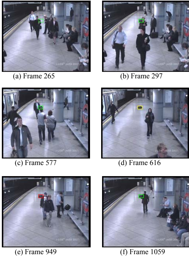
Figure 5: Results of processing sequence AB_medium . Figure 5(d) shows the identified unattended bag, which initiated reverse traversal up to Figure 5(a) where the bag was not found. Tracking in forward direction to Figure 5(b) re-discovered the bag and candidate owners were recorded. Figure 5(c) shows the point where the timer was set. 60s later, the alarm goes off in Figure 5(e) and is eventually discontinued in Figure 5(f) when the owner re-enters the scene.
